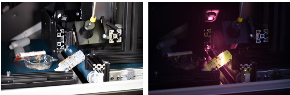
Fig. 4: Marked, dirty packages passing through the laser curtain with (left) and without (right) ambient light
