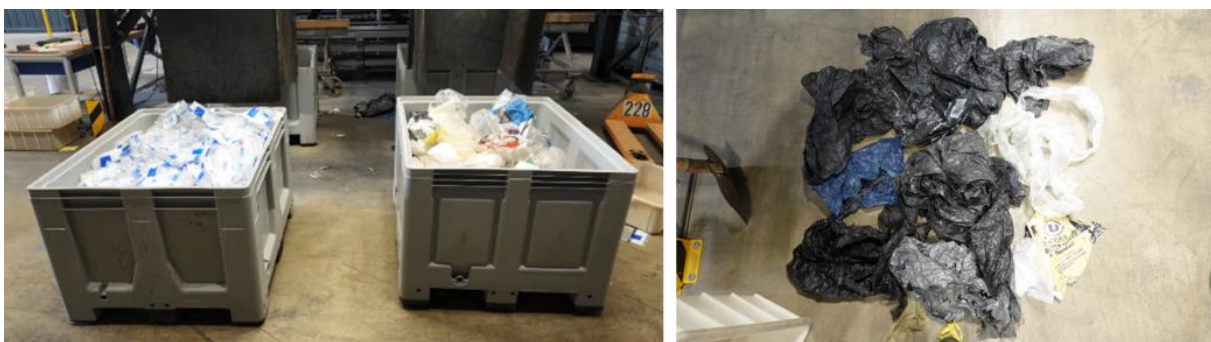
Fig. 6: Sorted fractions (left) and analyzed impurities (right) with a high proportion of black man-sized foils
