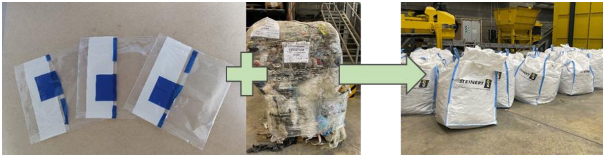
Fig. 5: Marked packaging pouches (left, 25 \mu\text{g}/\text{cm}^2 tracer in white ink) are mixed with household waste (center)
